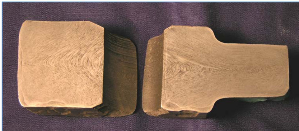
Macrograph showing the grain flow lines in a forged component
