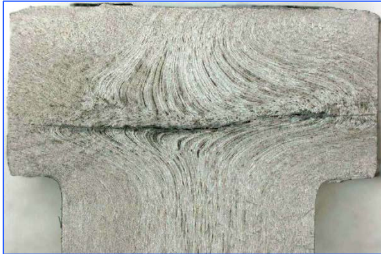
Macrograph of a forging burst
