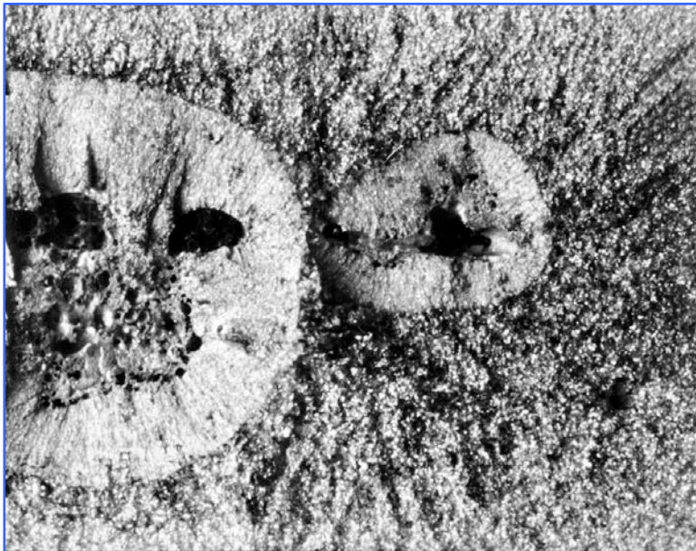
Fish eyes are bright patches named for their appearance on fracture surfaces
